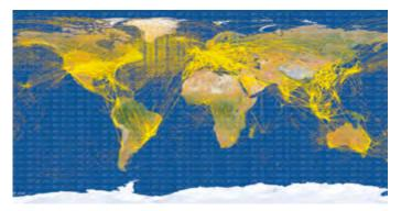
Apart from monitoring vegetation growth over Earth, the Proba-V minisatellite has recorded over 25 million positions from more than 15 000 separate aircraft. This is a technical world-first, demonstrating the feasibility of follow-on orbital constellations now being readied for operational aircraft monitoring
