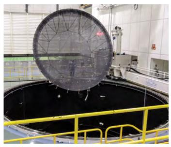
LABUM 5 m aperture demonstrator entering the Large Space Simulator
