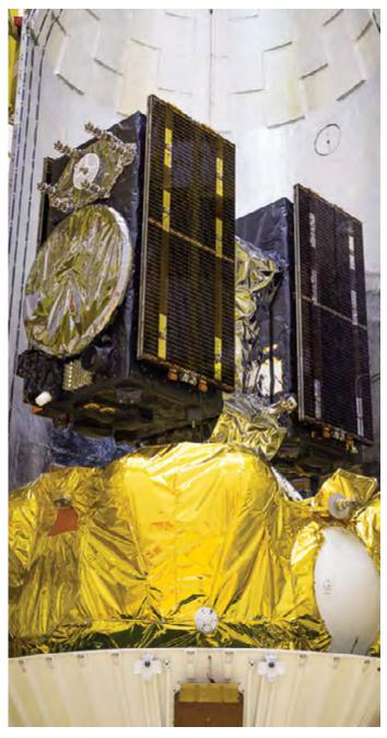
Galileo FM 08 and 09, mated with their dispenser on top of their Fregat upper stage being encapsulated within their Soyuz fairing, ready for launch on 17 December (ESA/ CNES/Arianespace/Optique vidéo du CSG/JM Guillon)
