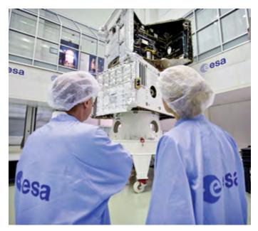
Europe's BepiColombo Mercury Planetary Orbiter seen atop its carrier vehicle, the Mercury Transfer Module, at ESTEC in 2015
